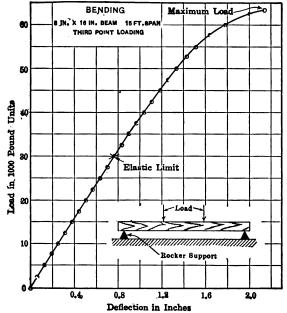
Fig. 3a.—Stress strain diagram for bending test.
